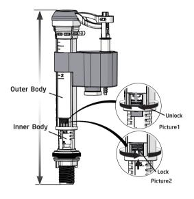
3.After the fill valve installed, unlock the outer Body in right direction. Adjust the height of fill valve (picture 1) to suitable level. Then lock again (picture 2);
