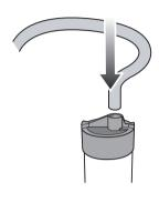
2.Connect the refill tube with refill rest-rictor from fill valve to the overflow pipe of the flush valve:
