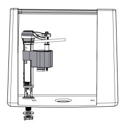
1.Insert the new fill valve with rubber seal at the base in the inlet hole of water tank and screw on the nut with collar tightly;
