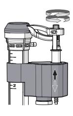
4.Fine and final adjustment can be made by rotating the screw rod clockwise or counterclockwise on the fill valve cup. In order to achieve desired water level;
