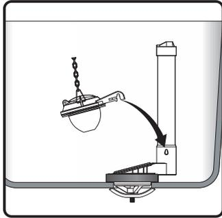
4. Connect the flapper to flush valve.
