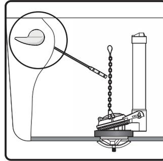
5. On the basis of form a complete set of lever installation instructions, install the tank lever in the toilet water tank corresponding assembly position.
