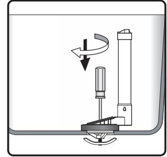
3. Tighten the bolt onto the "U" shaped hook by screw driver, make sure the flush valve is fixed properly.
