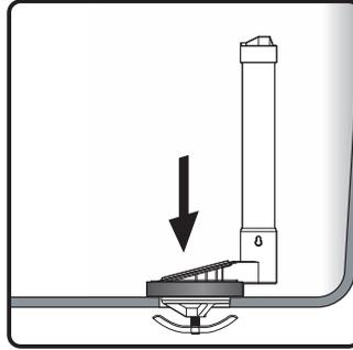
2. Position flush valve into the mounting hole.
