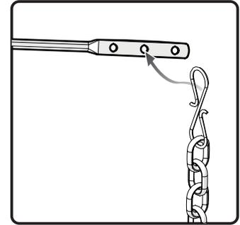
6. Connect the flapper chain. Allow slight slack when flapper is in closed position.
