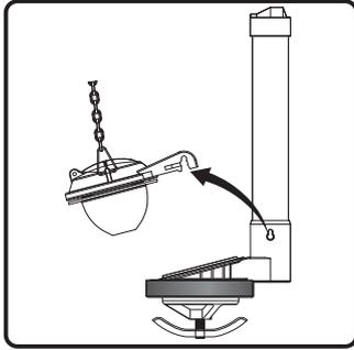
1. Disconnect the flapper from the flush valve.
